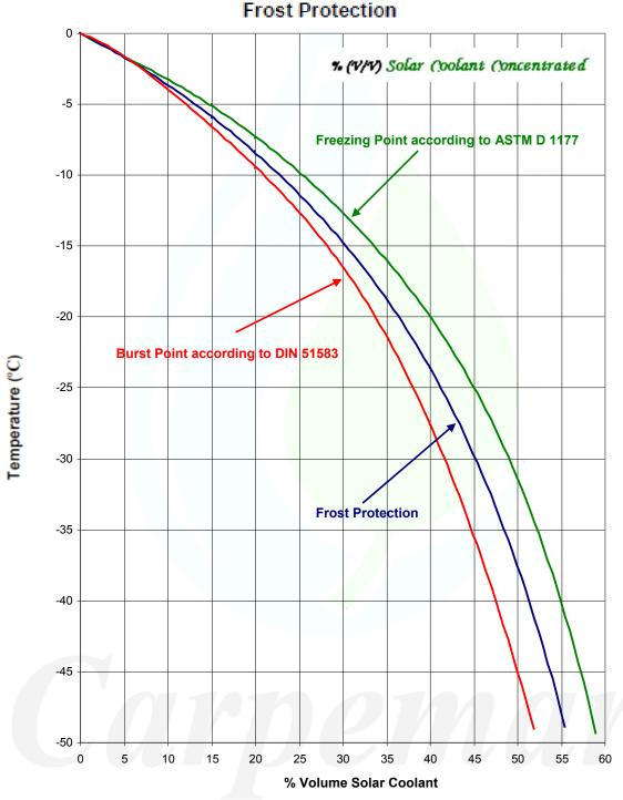
Freezing point according to ASTM D 1177 is the temperature for the first ice crystal formation.
